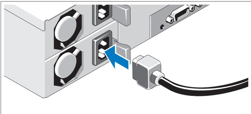
Connect the system's power cable(s) to the system and, if a monitor is used, connect the monitor's power cable to the monitor. Plug the other end of the power cables into a grounded electrical outlet or a separate power source such as an uninterruptible power supply (UPS) or a power distribution unit (PDU).
